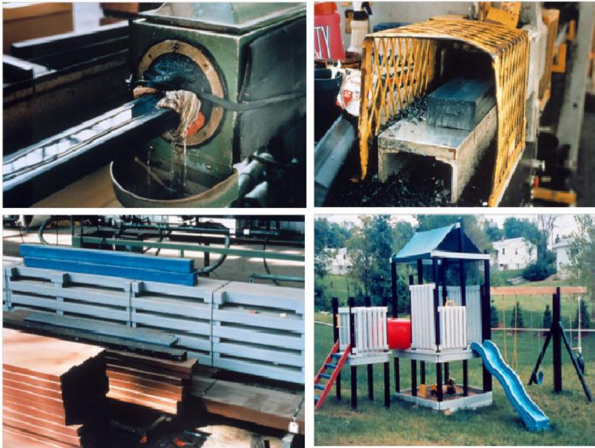
Figure 4. Recycling of HDPE into plastic lumber
