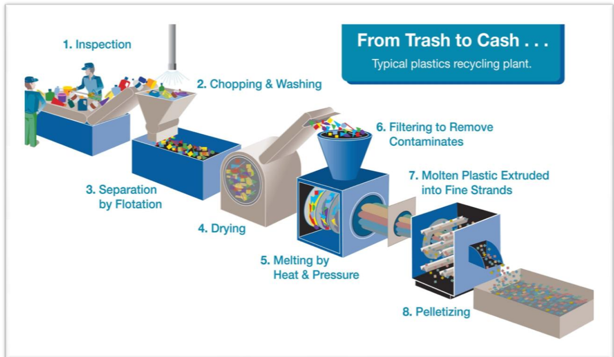
Figure 2. Plastic recycling process
