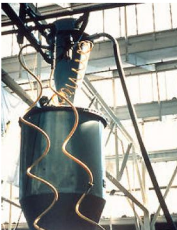
Figure 3. Container for melting of HDPE flake
